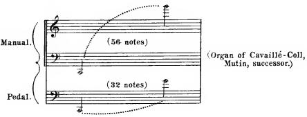
It would be highly desirable that organ-builders should come to an agreement on this point. No harm comes of the precise upper limit of the manuals being undetermined; the danger lies in the compass of the pedal-board varying from one Organ to another, for an organist should never need to look down at his feet when playing: his guiding-marks should be invariable, otherwise he treads on the wrong key.
